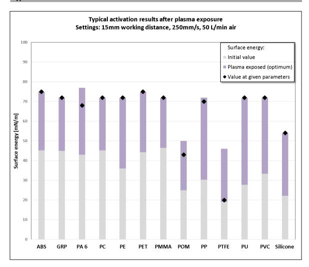
**A350** typical activation results for the given parameter set of speed and working distance operating with air. Higher surface energies through process parameter fitting can be achieved.
