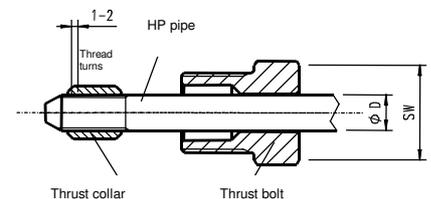
**Remark:** Prior to assembly (and if the medium permits such) all threads and sealing cones should be treated with a suitable lubricant (e.g. copper paste)!
