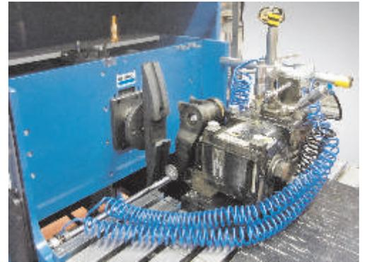
Brake testing machine with a fixture for a chockblock unit
