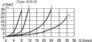
Q = f (s, x) Volume flow-signal-characteristics ( $\Delta p = 10 \text{ bar}$ ) [Type: ACB-S] Q [l/min]
