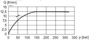
Q = f (s, x) Volume flow-signal-characteristics (Δp = 10 bar)
