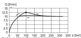
Q = f (s, x) Volume flow-signal-characteristics (Δp = 10 bar)
