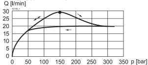
Q = f (p) Volume flow pressure characteristics [Type: V4D42-04] S = 100 %
