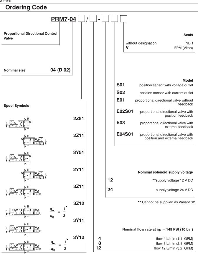
\* Model for cylinders with asymmetric piston rod, piston area ratio 1:2
