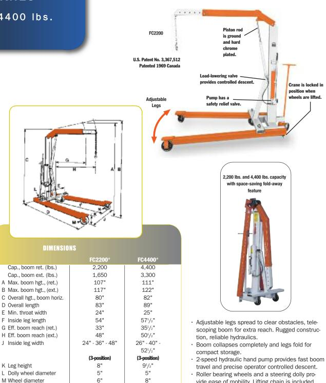
vide ease of mobility. Lifting chain is included. No. FC4400 - 4,400 lbs. cap. crane with fold-away feature, adj. leg spread, lifting chain and 2-speed hand pump. Wt., 646 lbs.
