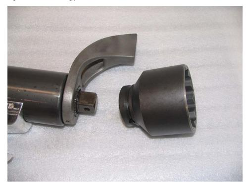
• Install the socket locking pin and retaining ring.
