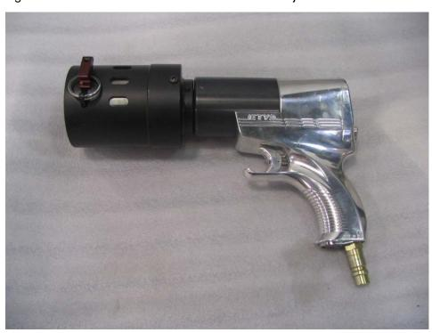
Figure 24. HYTORC Washer Socket Mounted on jGun
