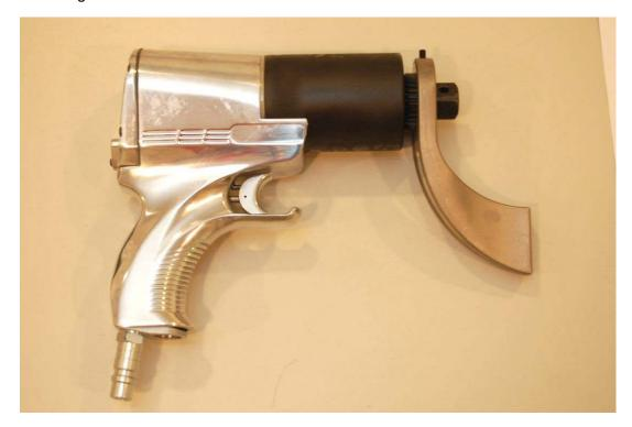
• Lock the reaction arm to the jGun by aligning the set-screw with the hole in the splined section and then tightening the set screw firmly.
