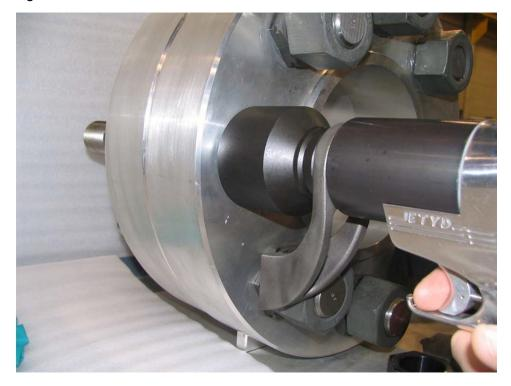
■ Using the HYTORC Washer <sup>TM</sup> eliminates external moving parts and increases worker safety. Refer to <u>HYTORC Reaction Washer Overview</u>.
