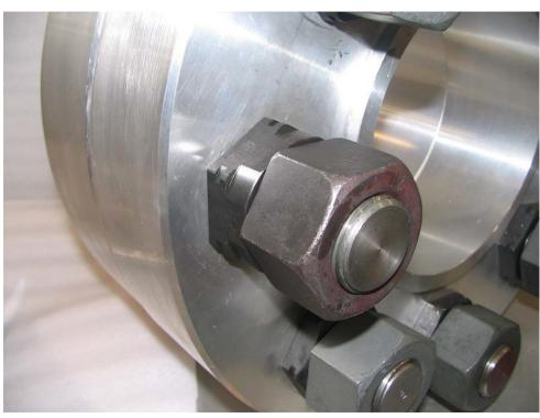
Figure 25. HYTORC Washer Installed
