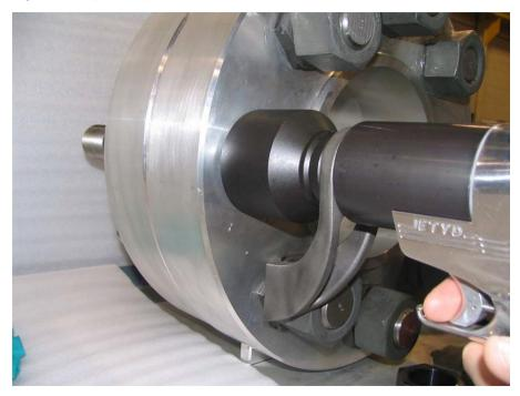
7. Torque the fastener by depressing the trigger until socket stops turning and air bypasses the motor.
