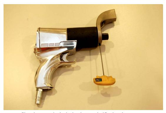
Place the appropriately sized socket onto the jGun barrel.
