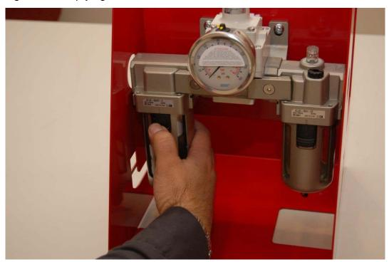
Figure 18. Emptying the FRL Filter Reservoir
