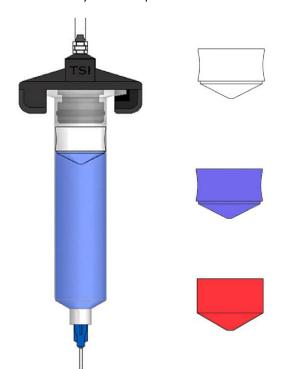
The tighter fit wiper pistons are recommended for use with low viscosity fluids and mechanical devices, such as a manual syringe gun, to prevent leakage past the double wiping edges.
