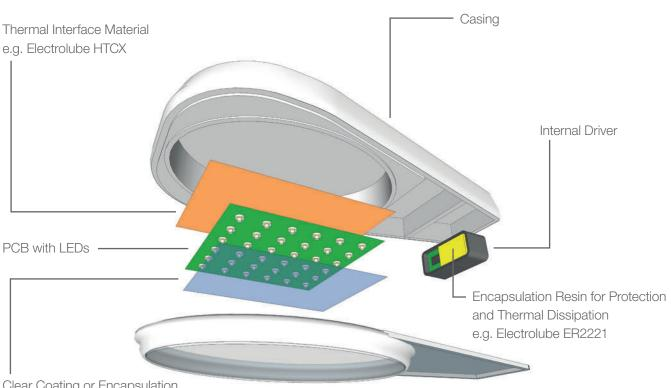
Clear Coating or Encapsulation Resin for Environmental Protection e.g. Electrolube AFA, UR5634
