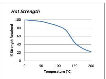
"Hot strength" shear strength tests performed on mild steel. Fully cured then conditioned to pull temperature for 30 minutes before testing. ES550 can withstand higher temperatures for brief periods (such as for paint baking and wave soldering processes) providing the joint is not unduly stressed.
