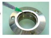
The two components can also be applied separately to a workpiece, so that curing sets in only after joining.
