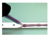
Most commonly, the adhesive is dispensed directly from the double cartridge or bead-on-bead with a dispensing gun. More precise dispensing is possible with a dispensing tip.
